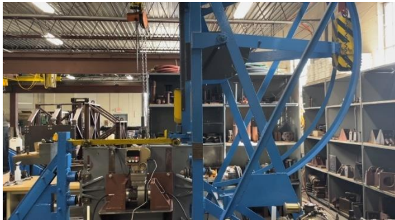
Figure 4: NPS 1.5 DDV in the Lightweight Shock Test Fixture per MIL-DTL-901E
