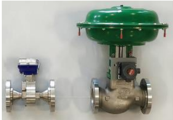
Figure 9: Two ANSI pressure class 150, 4" valves side by side. DDV shown left and Globe valve shown right.
